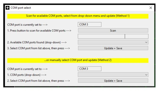
Follow the on-screen prompts in sequence (for either 'Method 1' or 'Method 2') to find and select the appropriate COM port and save your selection. When you have finished, either close the pop-up window or click the main window (the pop-up will close automatically).
